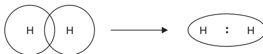
Fig. 2.3 Formation of \text{H}_2 molecule by the overlapping of two 1s atomic orbitals of two H atoms.
