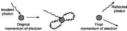
Fig. 3.8 : An electron cannot be observed without changing its momentum by an indeterminate amount
